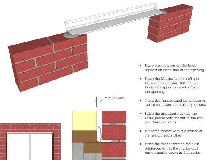
Place a supporting post c/c 1 m under the lintel/profile until the brickwork is hardening. The backside of the lintel is 20 mm, therefore there must be enough space between the brickwall and the supporting wall, se fig above.
